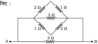
Calculate the equivalent resistance between the points A and B in the given Figure :
