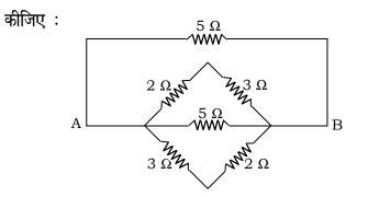
Calculate the equivalent resistance between the points A and B in the given Figure.
