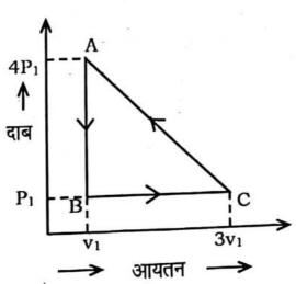
A gas is carried through the path AB, BC and CA according to the adjoining figure. What is the net work done in the whole cycle?
