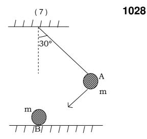
The bob A of a pendulum released from 30° to the vertical hits another bob B of the same mass at rest on a table as shown in Fig. How high does the bob A rise after the collision? Neglect the size of the bobs and assume the collision to be elastic.
