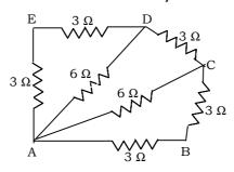
Find the total resistance between points A and B in the combination of resistances as shown in figure.
