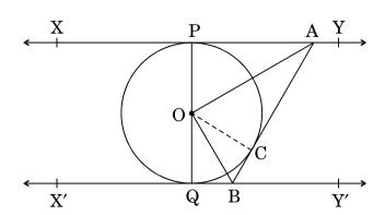
In the given figure, XY and X'Y' are two parallel tangents to a circle with centre O and another tangent AB with point of contact C, is intersecting XY at A and X'Y' at B. Prove that  $\angle$  AOB = 90°.
