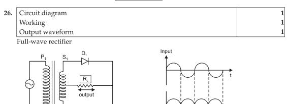
$\begin{array}{c|c} & & & \\ \hline & & \\ P_2 & S_2 & & \\ D_2 & & \\ \hline & & \\ During +ve half cycle diode D_1 is forward biased and diode D_2 is reverse biased. The forward current flows due to D_1. During -ve half cycle, diode D_1 is reverse biased and \\ \end{array}$
