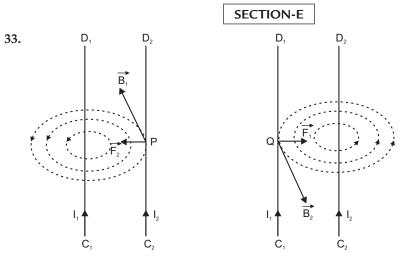
Consider  $C_1 D_1$  and  $C_2 D_2$  two infinite long straight conductors carrying currents  $I_1$  and  $I_2$  in same direction, at a distance r apart held  $||^{el}$  to each other. Mag. field Induction at pt. P on  $C_2 D_2$  due to current  $I_1$  in  $C_1 D_1$ .
