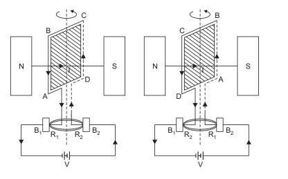
**Working:** As the armature coil is rotated in the mag. field angle  $\theta$  b/w field and normal to the coil changes continuously. An emf is induced in the coil. The direction of induced current is shown in figure.
