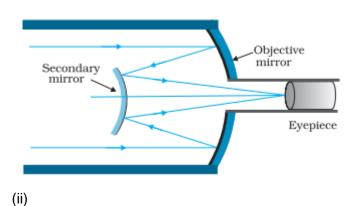
It has mirror objective, which is free from chromatic and spherical aberrations.
