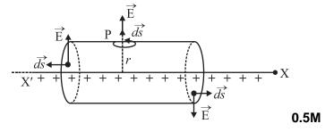
$\phi = \oint \vec{E} \cdot \vec{ds} = \int_{LCF} \vec{E} \cdot \vec{ds} + \int_{CS} \vec{E} \cdot \vec{ds} + \int_{RCF} \vec{E} \cdot \vec{ds} \mathbf{0.5M}$ =  $\int_{LCF} Eds \cos 9 \, 0^\circ + \int_{CS} Eds \cos 0^\circ + \int_{RCF} Eds \cos 9 \, 0^\circ \mathbf{0.5M}$  $\phi = \int_{CS} Eds \cos 0^\circ = E \cdot 2\pi rl \qquad \dots (1)$
