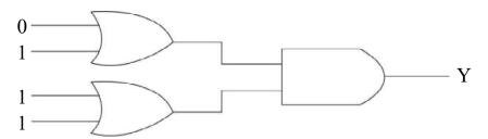
Write value of output Y in diagram.
