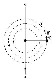
$\operatorname{dir}^n$  of  $\stackrel{\rightarrow}{B}$  is along the tangent to mag. field line at that point.
