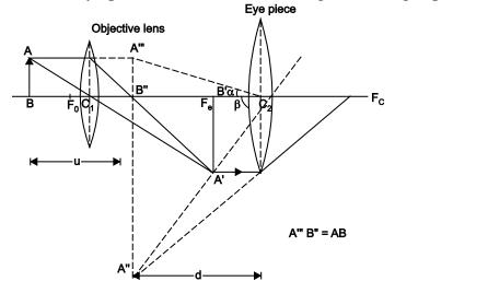
Magnifying power of compound microscope is defined as ratio of angle subtended by final image and object on eye when both are at least distance of distinct vision.
