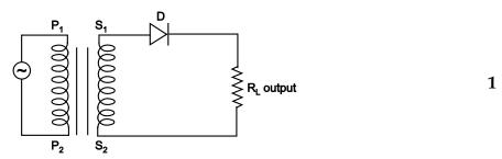
During the half cycle diode D is forward biased and forward current flows through the diode; we get output. During –ve half cycle diode D will be reverse biased hence will not conduct. The output waveform is shown in fig.  $\mathbf{1}$
