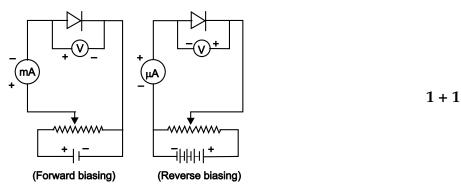
At some forward voltage *i.e.*, 0.7 V for *Si* and 0.3 V for *Ge* known as knee voltage the potential barrier is almost eliminated and the current starts flowing and curve rises sharply as shown in Fig.
