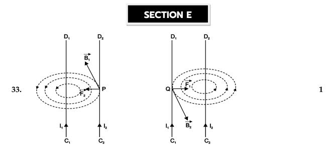
Consider  $C_1D_1$  and  $C_2D_2$  two infinite long straight conductors carrying currents  $I_1$  and  $I_2$  in same direction at a distance *r* apart held  $\parallel^{el}$  to each other.
