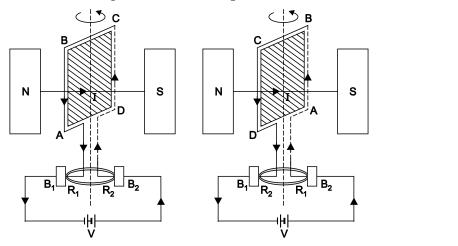
**Working:** As the armature coil is rotated in the mag. field angle  $\theta$  b/w field and normal to the coil changes continuously. An emf is induced in the coil. The direction of induced current is shown in figure.
