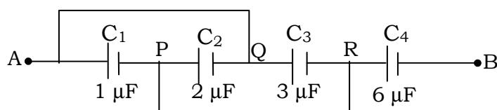
Calculate the equivalent capacitance between the points A and B in the following Figure :
